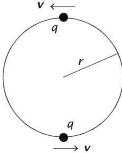
Figure 4: Two identical charges moving on the same circle at diametrically opposite points. This system has zero dipole moment and will radiate only quadrupole radiation.
